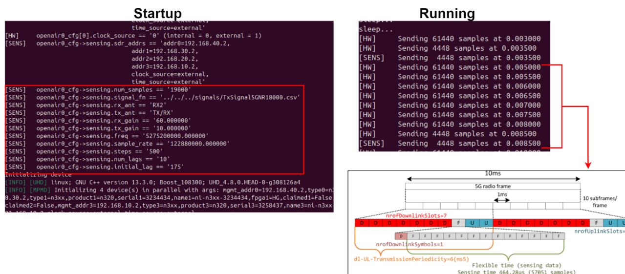
Figure 3-3 Execution example of the Sub-6 gNB with sensing capabilities
