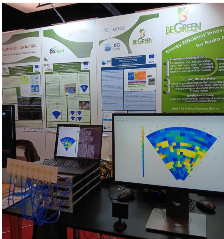
Figure 3-5 Sub-6 GHz ISAC Prototype with 6G-SENSES E2SM for sensing
