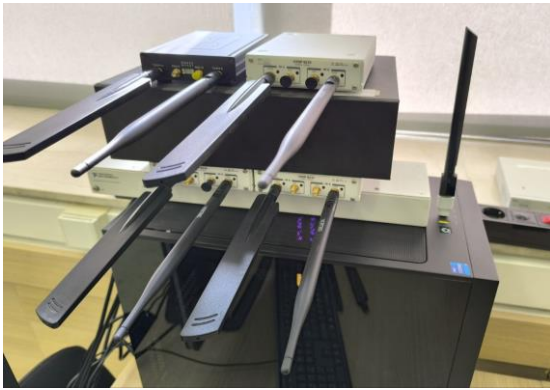
Figure 4-22 USRP-based 2x2 MIMO testbed (Front view), USRP-based 2x2 MIMO testbed (Rear view)
